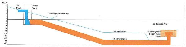
Figure 5: Preliminary Hydraulic Profile of Suction Pipelines
