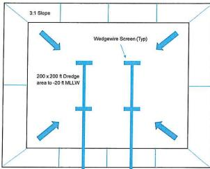
Figure 4: Wedgewire Sceen Arrangement in Dredged Area
