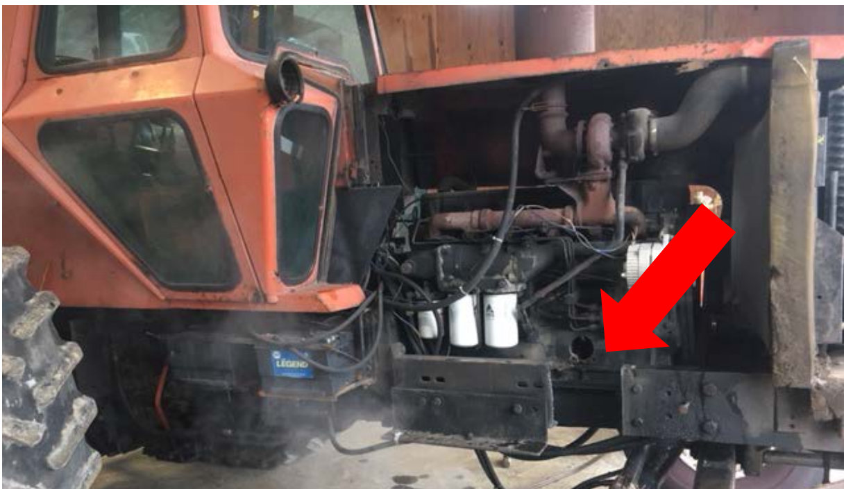
Figure 11. After Photo, with Frame Rail Cut
